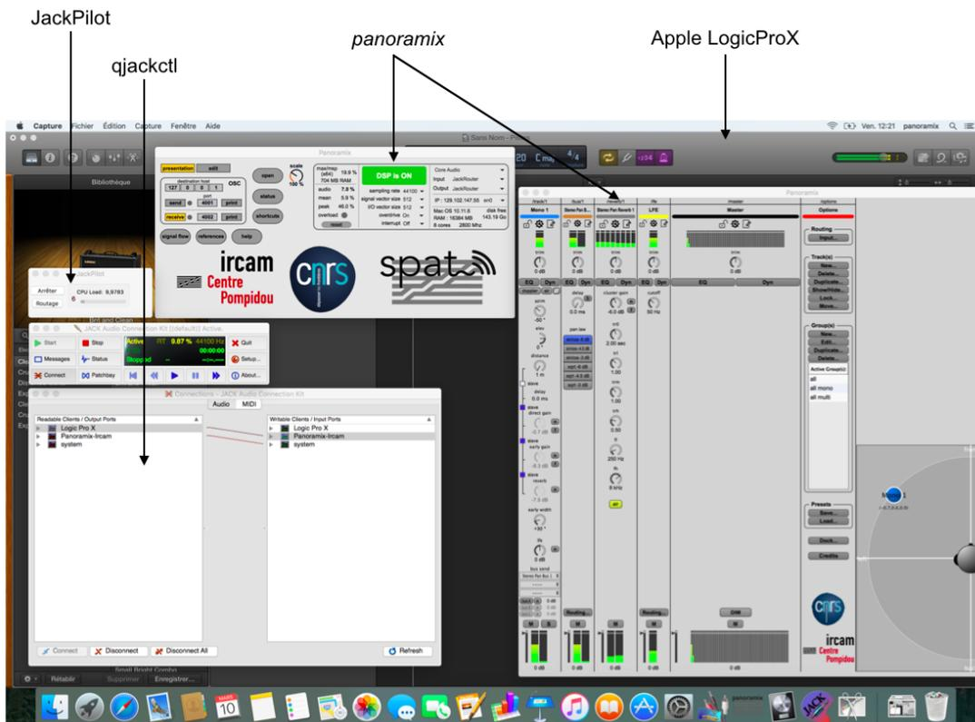
Figure 18: Virtual audio driver workflow: example with *panoramix* and LogicPro virtually connected through the JackPilot.
